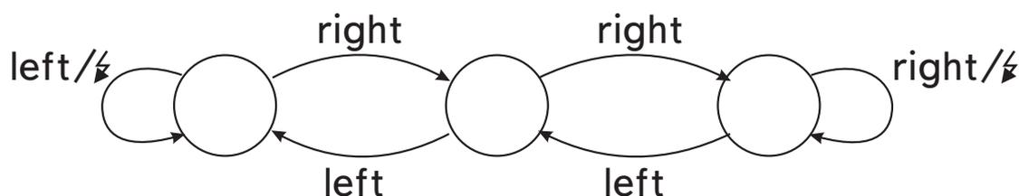
Fig. 3: The FSM which gives the "x" coordinate
