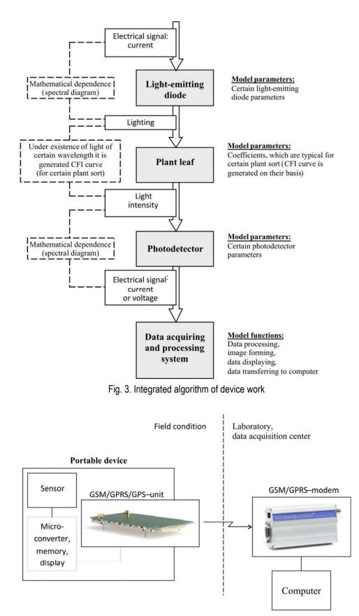
Fig. 4. Data acquiring, processing and transmitting system on the base of portable device with radio channel
