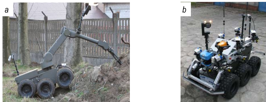
Figure 1. IBIS mobile robot: the commercial version (a), testbed version for autonomy method development (b)
