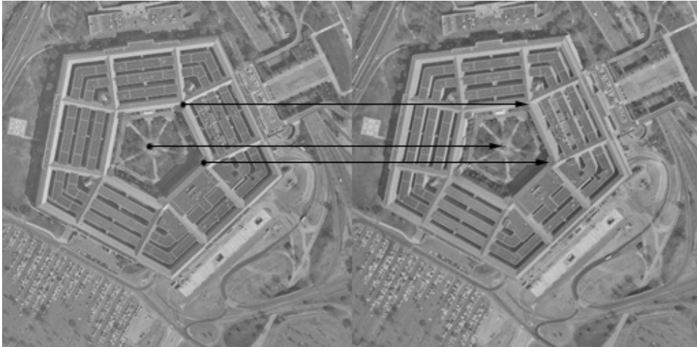
Figure 100. Point matching of the stereo pair of satellite images
