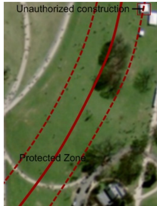
Figure 105. Automatic revealing of not authorised building in a security zone of the main gas pipeline with use of program complex ENVI
