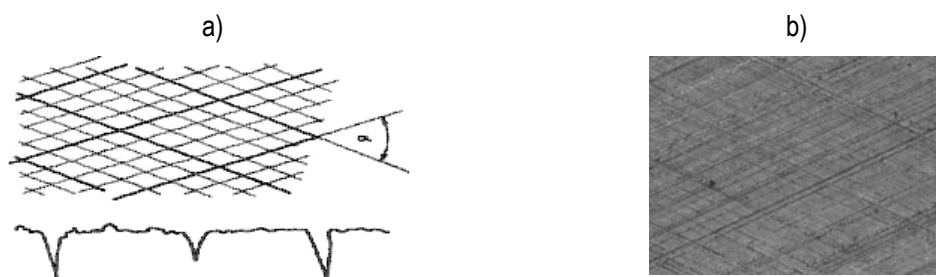
Fig.1 Schematic diagram of a cylinder after honing (a) [Zwierzycki, 1990] and a photograph of the surface of a cylinder liner (b)
