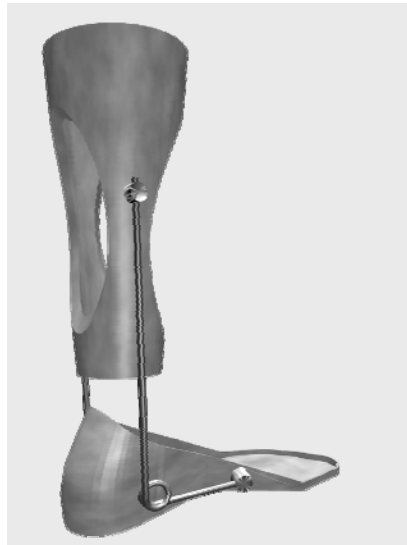
Fig.6. 3D computer solid model of MAFO in state of tension includes two parts: lower part (foot) and upper part (calf) with two torsion spring (lateral and medial).
