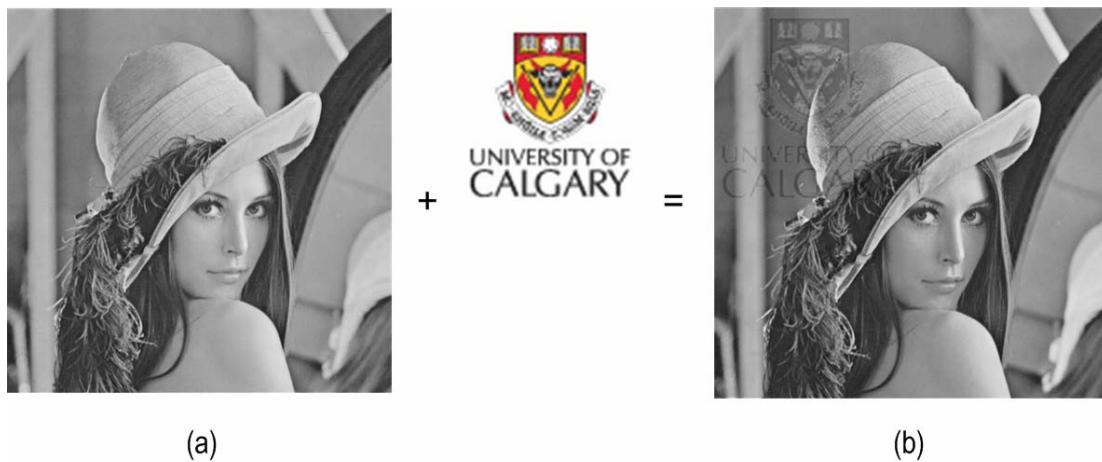
Figure 2. Examples of (a) the original image and (b) the image with embedded visible watermark
