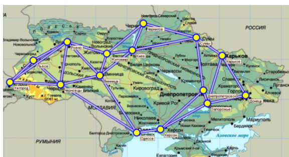
Figure 1 Initial MPLS network structure
