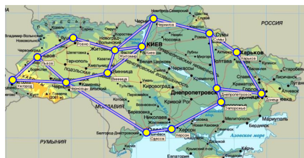
Figure 2 Optimized MPLS network structure
