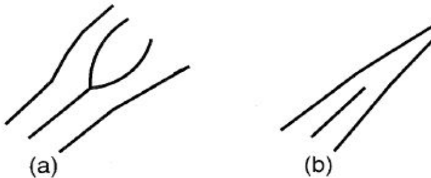
Figure 2. Features extracted from fingerprint: (a) ridge bifurcation; (b) ridge ending
