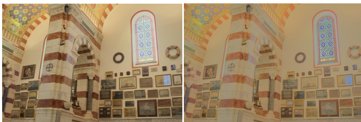
Figure 12 : Tone mapped images. (Left) Our modified tone mapping algorithm. (Right) Our original algorithm.
