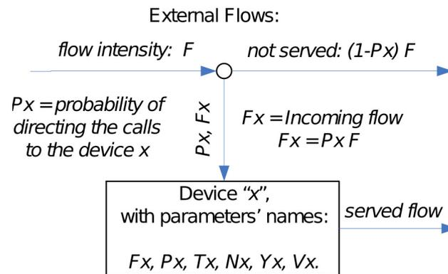
Figure 1: Graphical representation of a base virtual device.
