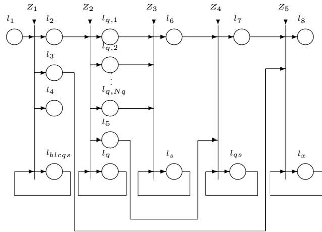
Figure 20: GN model of the simple causal structure representation of a queuing system.
