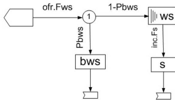
Figure 13: Classical conceptual model of a queuing system.
