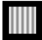
Fig.2 Measured object (simulation formula) O(x, y) = 1 + 0.3 \text{SIN}(kX)
