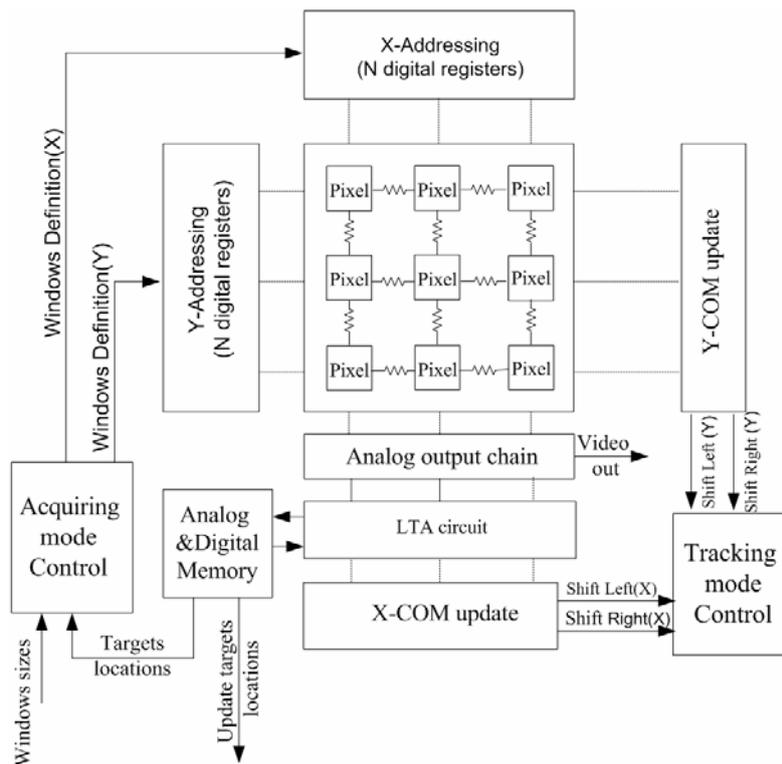
Figure 2. Architecture of the proposed tracking sensor.
