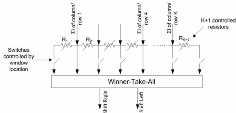
Figure 4. The X-COM and Y-COM update circuit implementation
