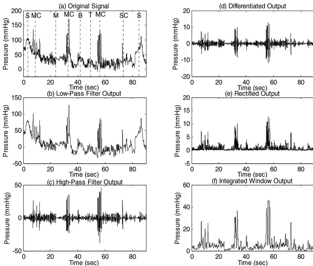
Figure 2 - Sample data of (a) original signal, (b) low-pass filter output, (c) high-pass filter output, (d) differentiated output, (e) rectified output, and (f) integrated window output.
