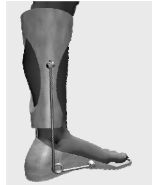
Fig.7. 3D model of the human ankle-foot segment with a model of orthoses.
