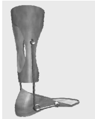
Fig.6. 3D computer solid model of MAFO in state of tension includes two parts: lower part (foot) and upper part (calf) with two torsion spring (lateral and medial).
