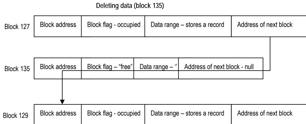
Fig. 2 Deleting data in block structures
