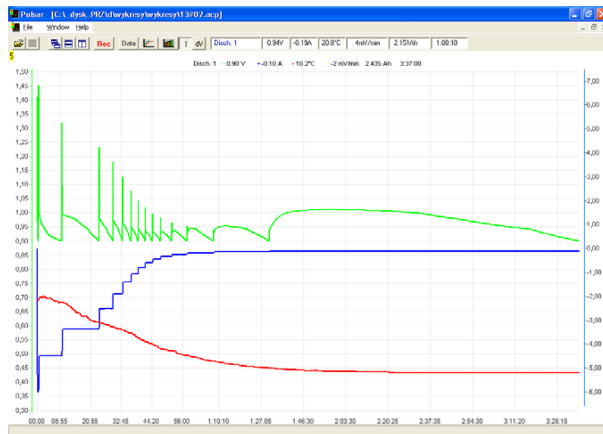
Fig. 16. Self-regeneration of a package during the charging process.
