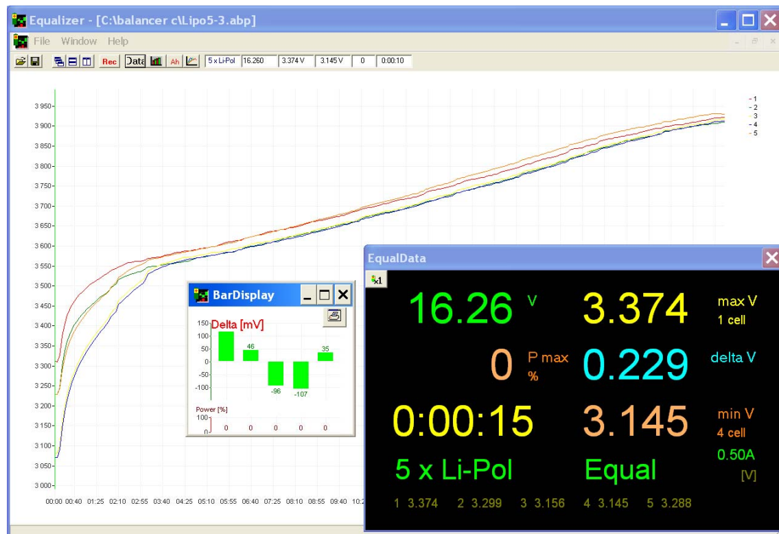
Fig. 24. The correct cycle of package leveling.
