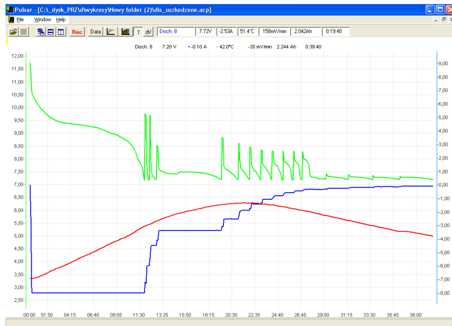
Fig. 11. The partial regeneration of the faulty cell during the discharging process.
