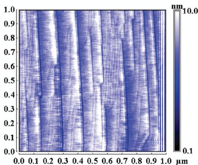
Figure 1 – AFM-image of the  $1.69^\circ$  off cut STO substrate
