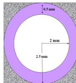
Figure 3 – Schematic representation of a superconducting ring 0.5 mm in diameter (purple area) on a 5.5 mm<sup>2</sup> YBCO thin film platelet with outer radius 2.5 mm and inner radius 2 mm
