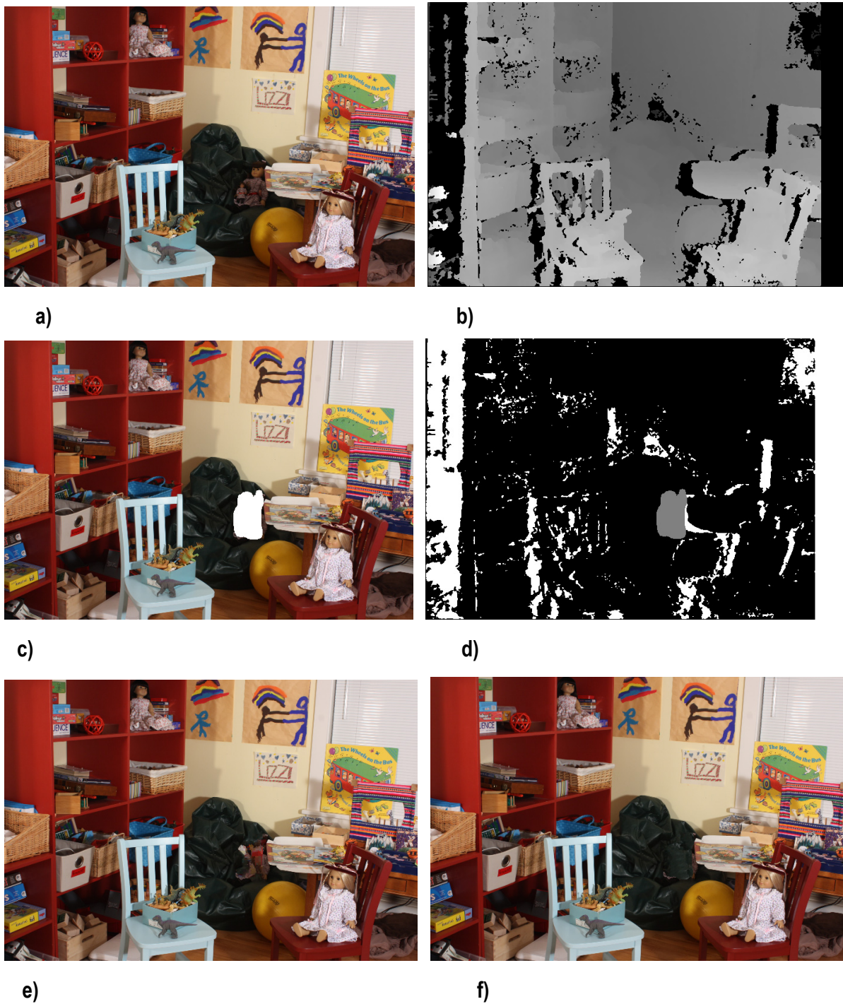
Figure 3: Example2. Comparison of exemplar based inpainting and our approach. Image size is 640x480, a) the original image , b) depth map, c) inpainted image d) inpainting mask, e) result of Criminisi's algorithm, f) our result
