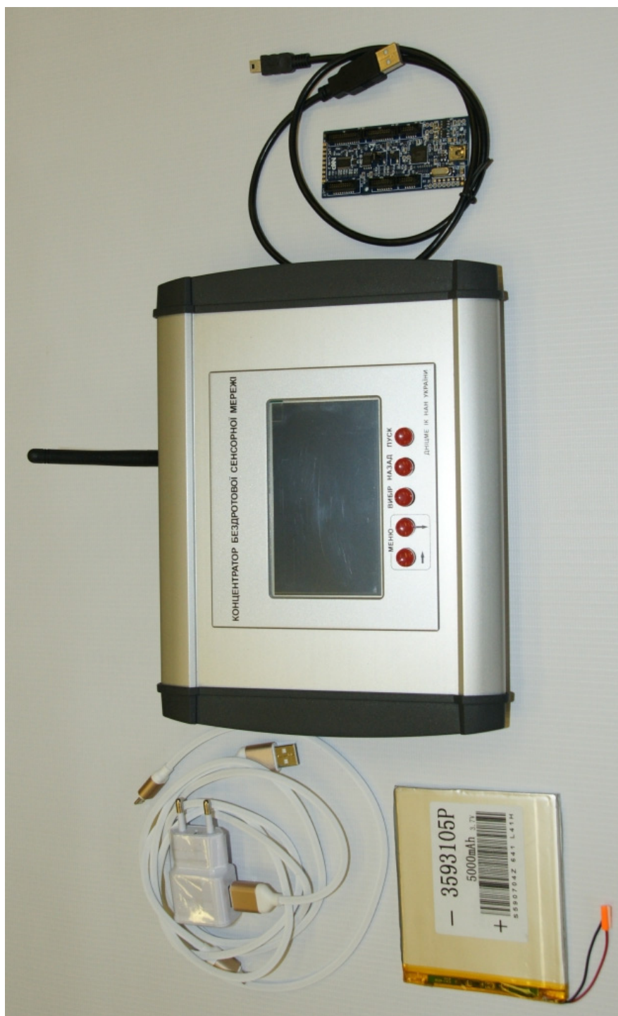
Fig. 7. Concentrator of network of sensors
