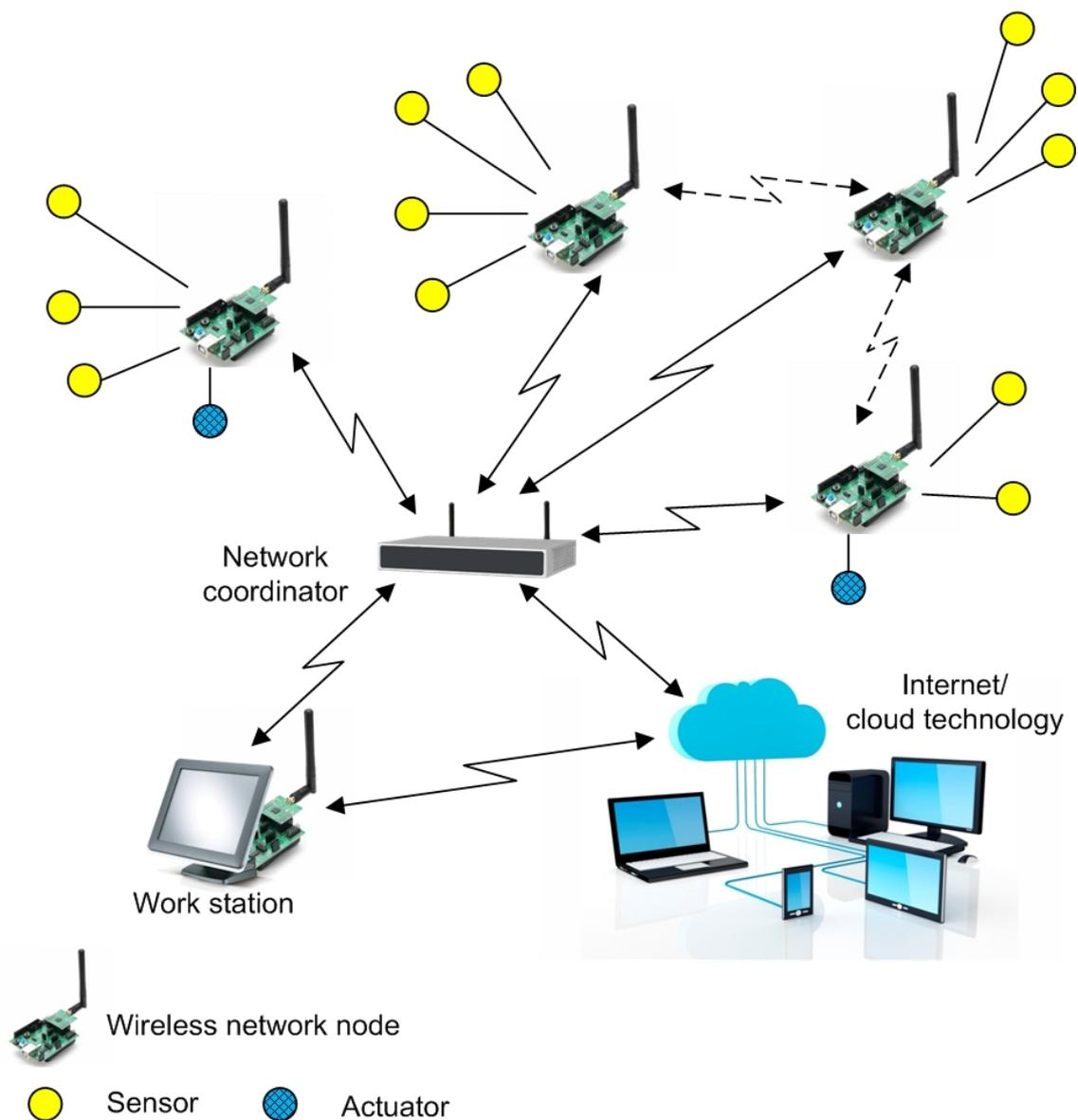
Figure 5. Architecture of type industrial WSN
