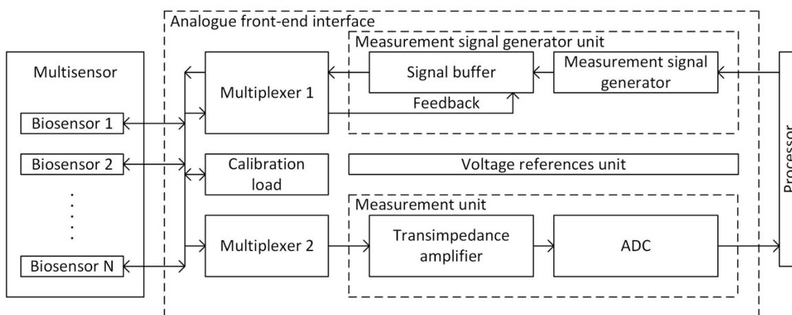
Figure 3. Analog front-end interface of smart multisensor node
