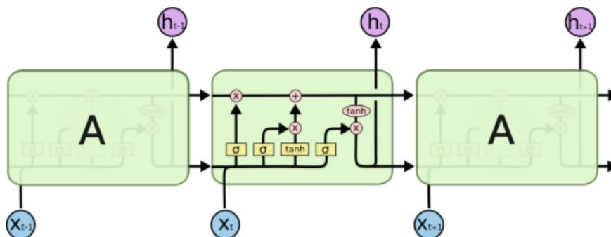
Figure 3. LSTM based RNN Architecture [Cohah 2015]
