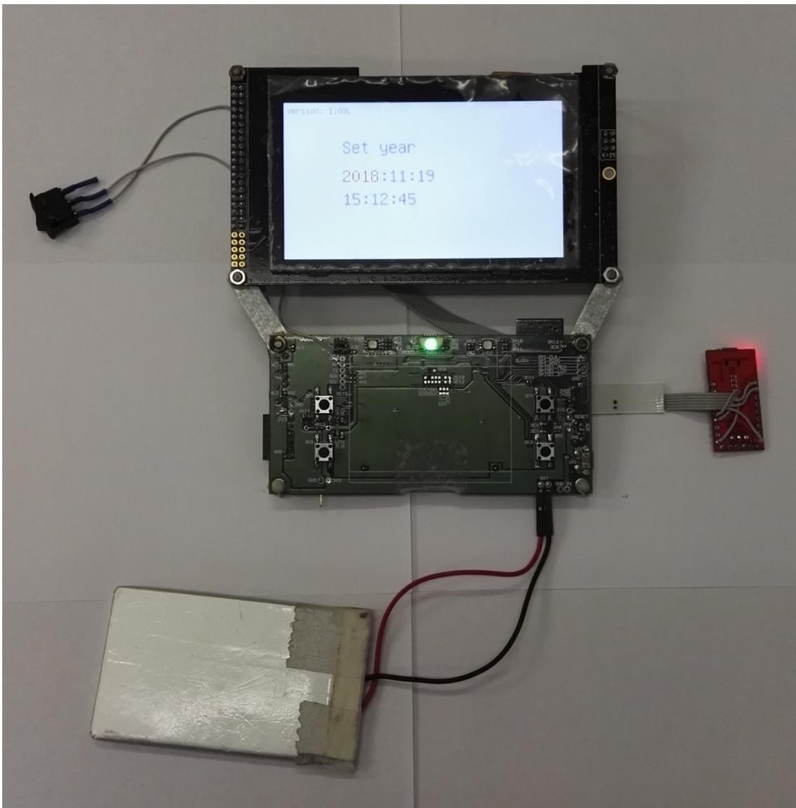
Figure 8. Prototype unit of WSN coordinator
