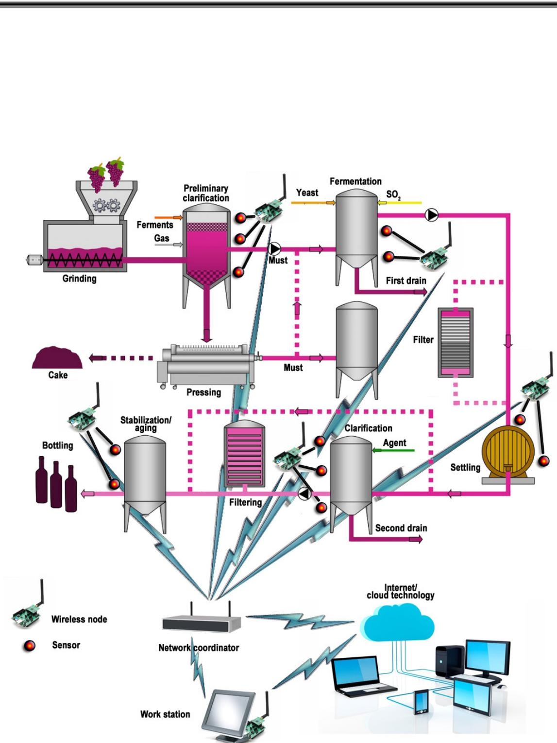
Figure 6. Architecture of WSN for application in industrial wine-making manufacture
