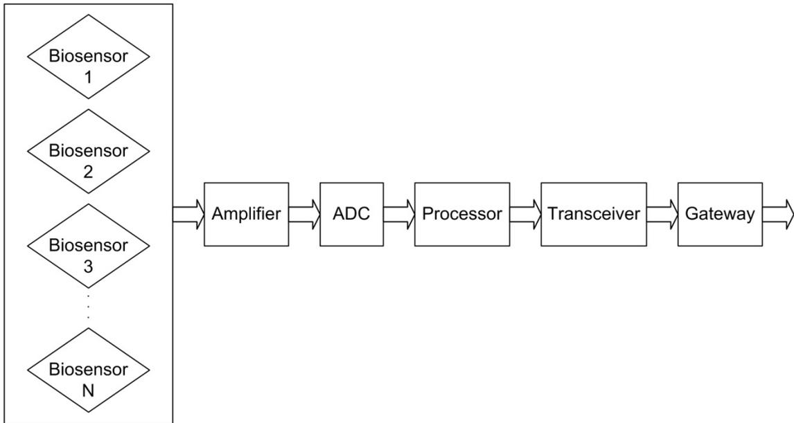
Figure 1. Block diagram of typical smart multisensor node
