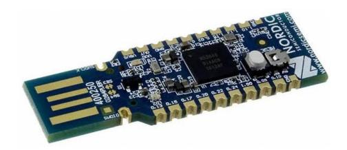
Figure 5. Wireless microcontroller nRF52840
