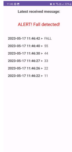
Figure 13. The smartphone has received the "FALL" message
