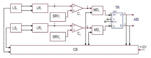
Fig.3. Structural scheme of the device for counting of bottles
