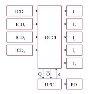
Fig.1 Structural diagram of automated system for counting of bottles on conveyor belt
