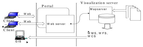
Fig. 3. Visualization system using thin client
