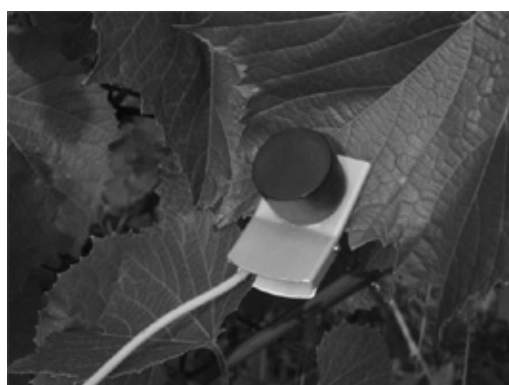
Figure 6. The sensor of the "Floratest" on the vine leaf and the image of CFI on the device's display
