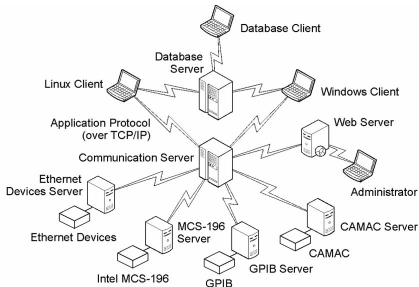
Figure 1. The scheme of the distributed information measurement and control system
