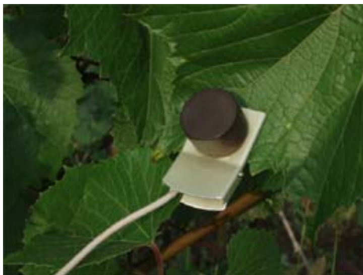
Fig. 8. The sensor of the "Floratest" on the vine leaf
