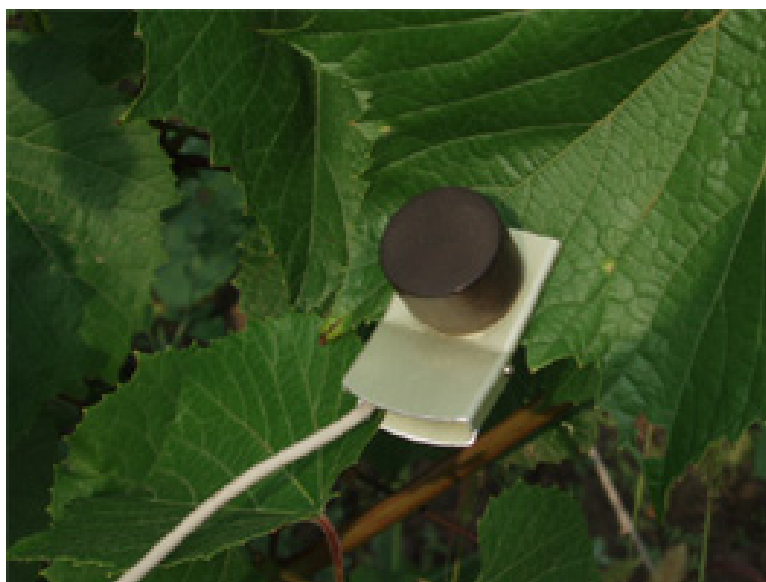
Fig. 8. The sensor of the "Floratest" on the vine leaf
