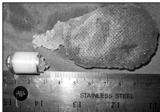
Fig. 9: Separated CE and stabilizing component.
