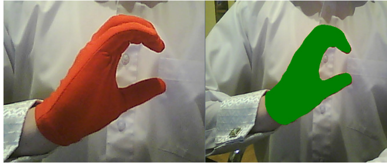
Figure 1. Image of gesture that is captured from a webcam. A contour of hand is found and highlighted
