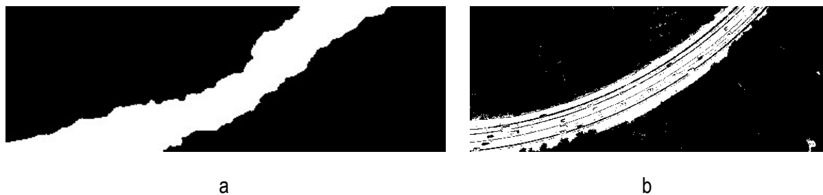
Fig. 2. Similarity map for chosen template (a) and binary pattern of the road (b).
